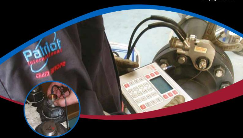
The USM II Ultrasonic Bolt Meter is an electronic device which is used to measure extremely accurately, the extension of a bolt of virtually any material from 25mm to 15 meters in length. The physics governing the process are clearly understood and have been employed for many years in the fields of
